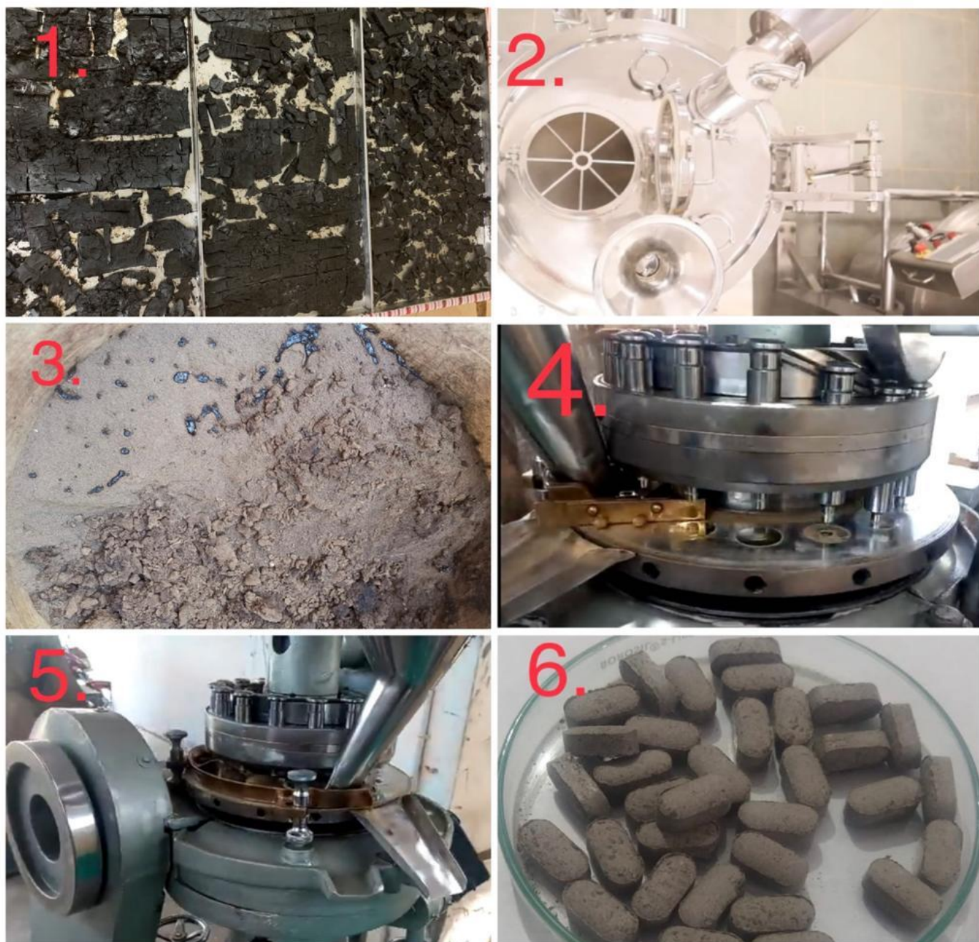
Fig. 1. Dried ghan , 2 & 3. Granule formation, 4 &5. Making tablet in tablet punching machine, 6. Final tablet
