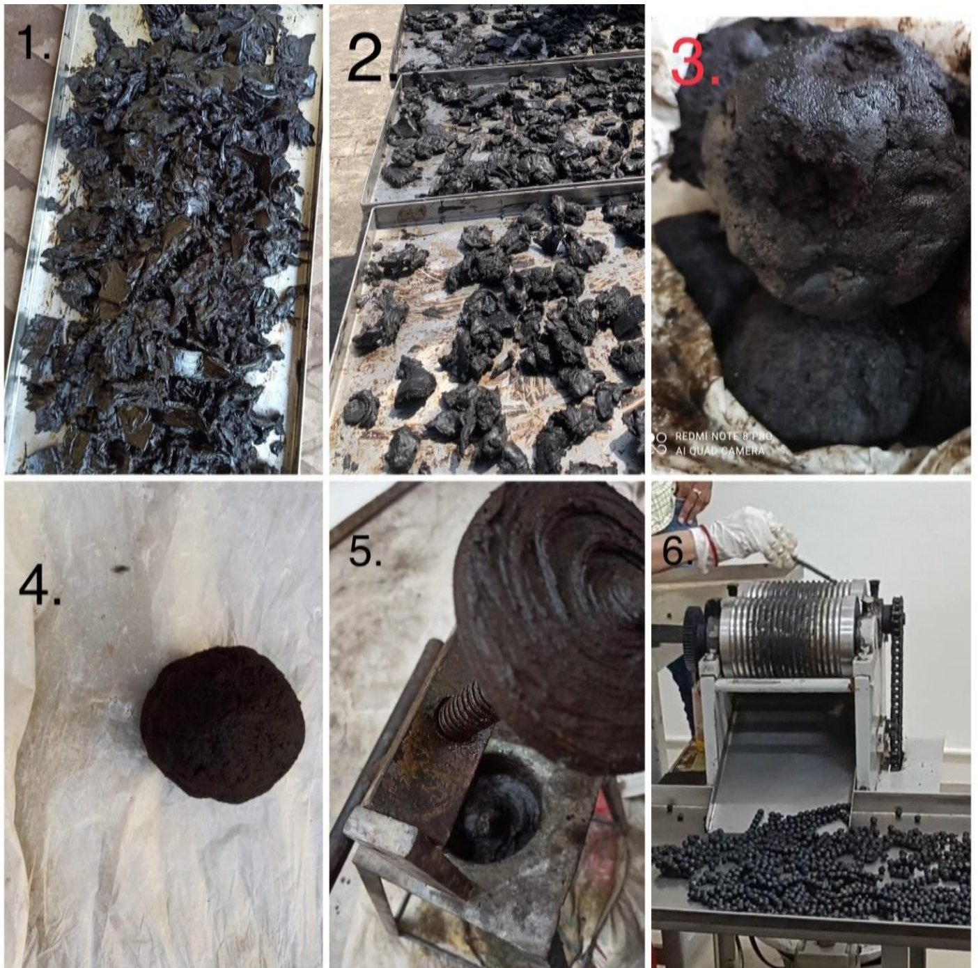
1&2. Dried ghana , 3&4. After pounding of ghana , 5. Making wicks in extruder, 6. Vati made in pill making machine.
