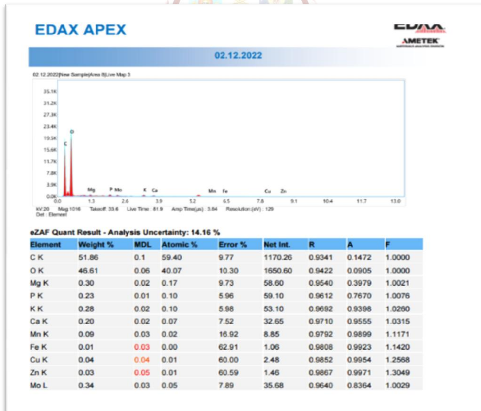
Figure 5: EDAX results of elemental composition with Carbon and oxygen at maximum
