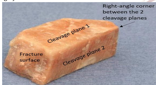
Fig.6 K-feldspar having two cleavage direction and Fracture surface
