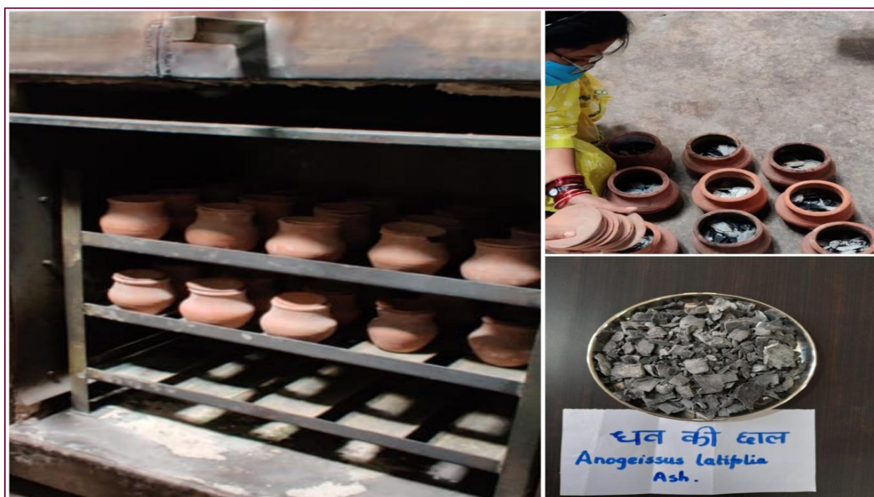
Preparation of Dhava ( Anogeissus latifolia Wall.) bark ash in Muffle Furnace
